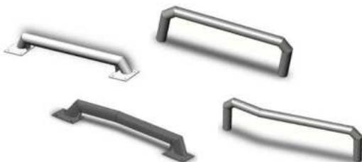
Wheel guides help the truck driver to reverse to the loading bay without any complicated maneuvering actions. They are installed on yard level, either by being cast directly into concrete (types PEK and PEKE) or by being bolted on the ground (types PEF and PEFE); they represent a good and reasonable investment into the safety at your loading bay.
