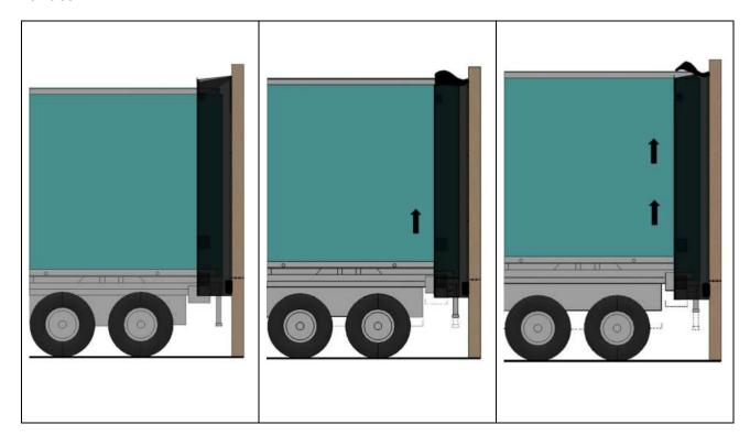
The vehicle is lifted after dock-in into the dock shelter. The roof automatically follows this movement and returns to its original position after the vehicle has left the docking station.
