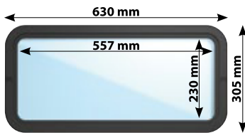
Rounded corners (r=60 mm), excellent insulative value
